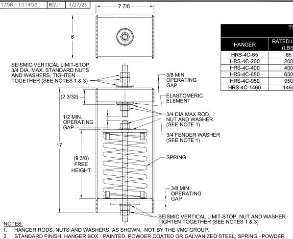
SEISMIC VERTICAL LIMIT-STOP REQUIRED FOR SEISMIC APPLICATIONS: NOT BY THE VMC GROUP. INSTALL
